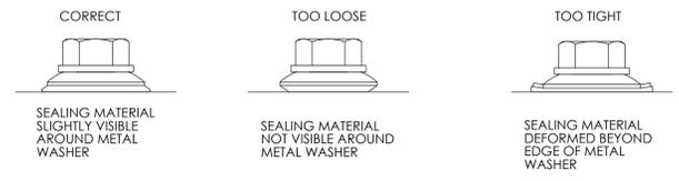
ROOF FASTENER TIGHTENING
