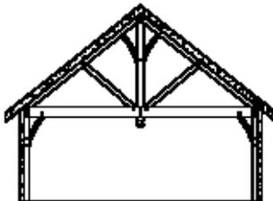
TIMBER FRAME WITH SIP WALLS AND ROOF
