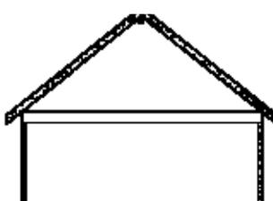
STORY AND A HALF WITH ENGINEERED FLOOR COLLAR TIE SIP WALLS AND ROOF
