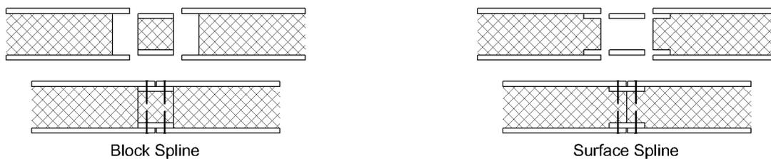
**Figure 1: SIP Spline Types**
