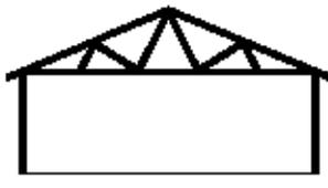
SIP WALLS WITH TRUSS ROOF
