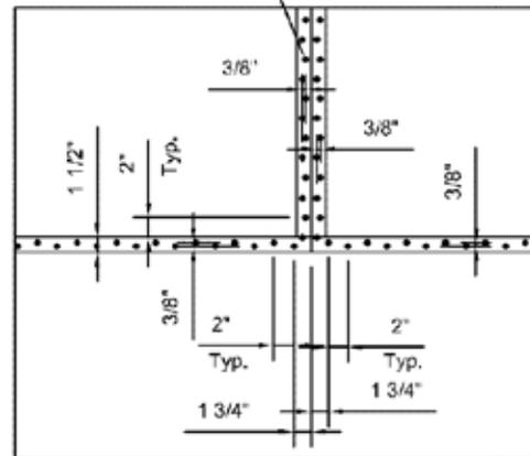
**Figure 3c: Boundary Spline**
